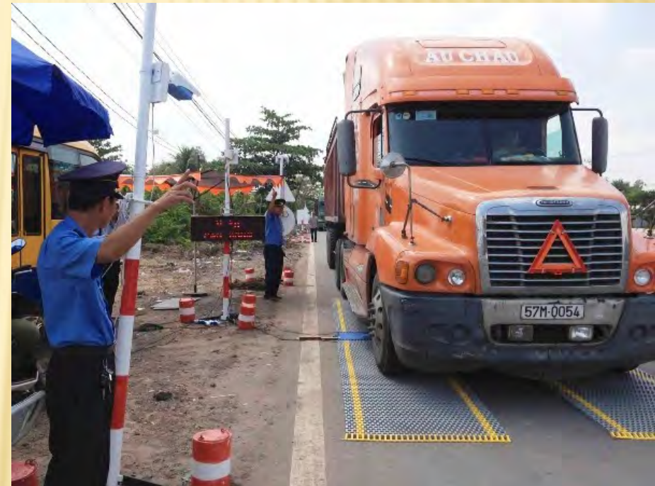
A truck being weighed on mobile truck scales
